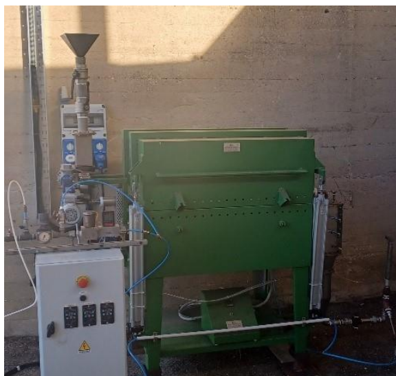
Figure 1 Rotary kiln reactor
