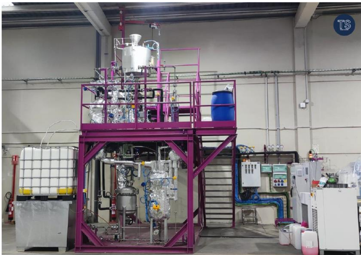
Figure 1 Microwave-assisted unsorted plastic waste pyrolysis pilot plant 1
